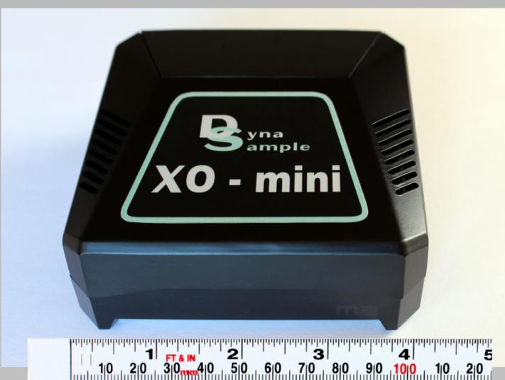
With a width of just a little over 4 inches (10 cm) and a weight of 280g it is small enough for carrying it on your body or even mount it on your wind controller when using battery power (5V - 3Ah USB C).
